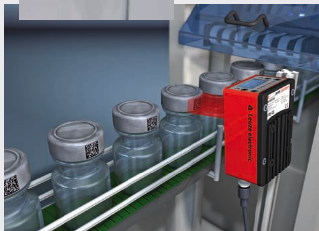
Presence inspection of caps and code reading
