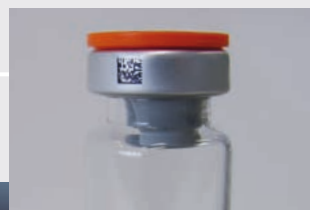
Presence inspection of caps and code reading
